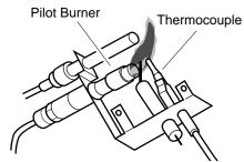
Figure 30 - Incorrect Pilot Flame Pattern
